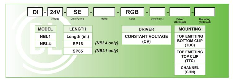
Example: DI-24V-SE-NBL4-RGB-16-CV-TBC = Diode LED, 24V NEON BLAZE<sup>TM</sup>, 4.44 w/ft. RGB, 16.4' long, 96" Lead Wire, and with a Constant Voltage Driver, and Top Emitting Bottom Clips.
